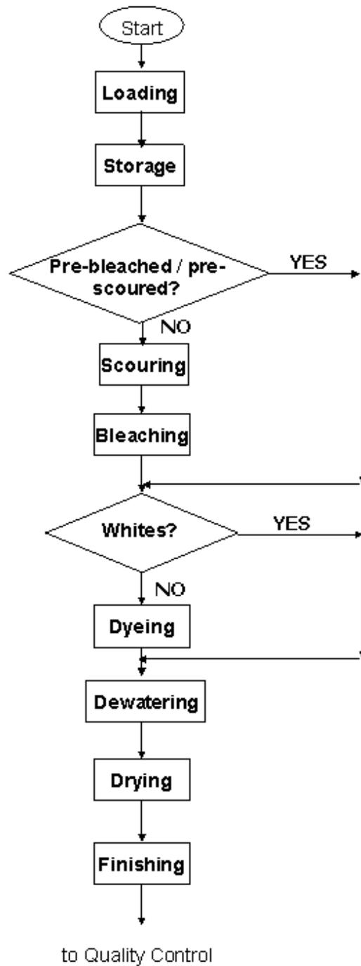
**Figure 4-3: A Flowchart Indicating a Process Operation in a Wet-textile Processing Unit for Special Situations**
