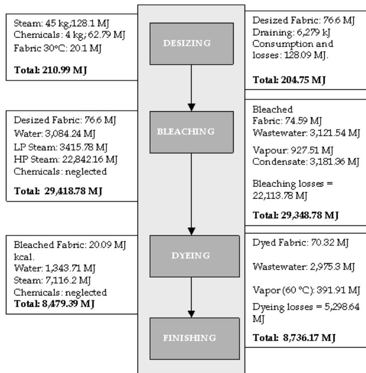
Figure 4-5: A Detailed Energy Balance in a Wet-textile Processing Unit
