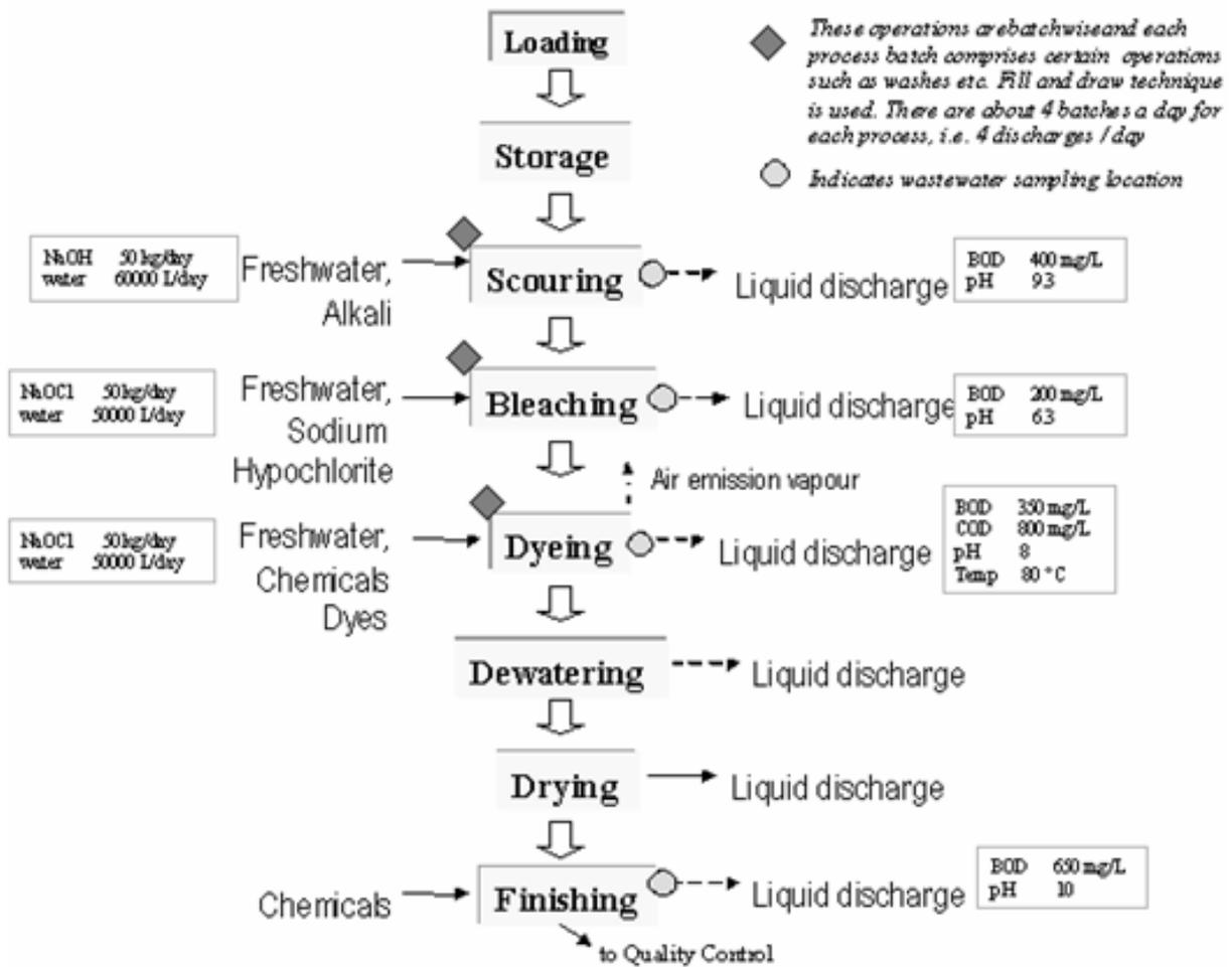
Figure 4-2: A PFD for a Wet-textile Processing Factory
