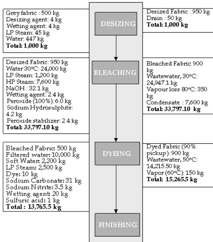
Figure 4-4: A Detailed Material Balance in a Wet-textile Processing Unit
