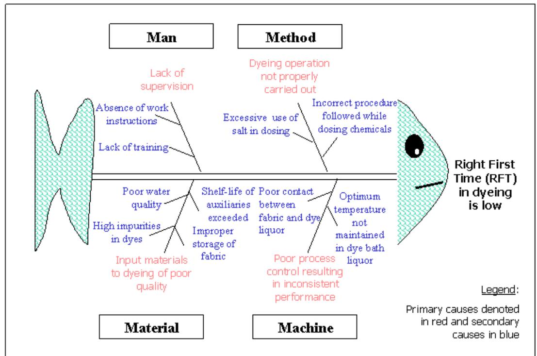
Figure 4-6: Illustration of a Fishbone Diagram to Facilitate Cause Diagnosis in the Dyeing Process
